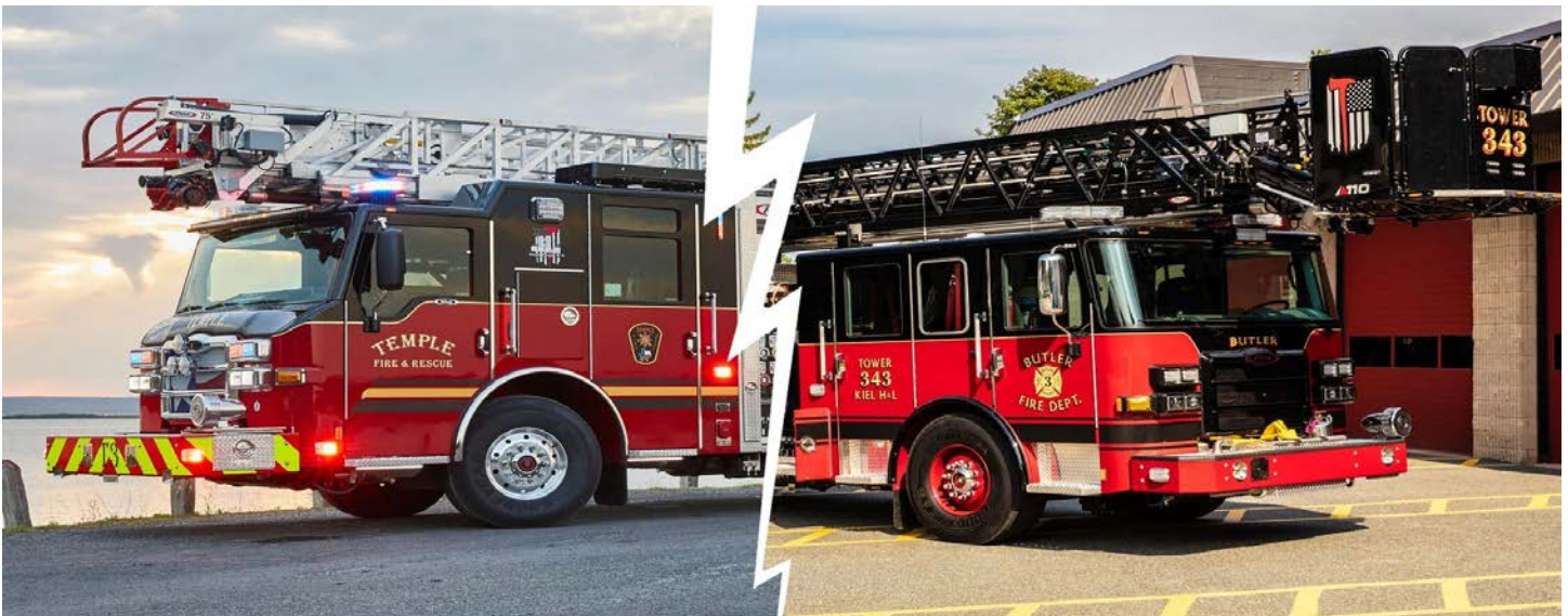
Photo to illustrate the difference between an aerial ladder (left side) and a platform aerial (right side)
