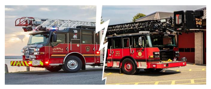
Photo to illustrate the difference between an aerial ladder (left side) and a platform aerial (right side)
